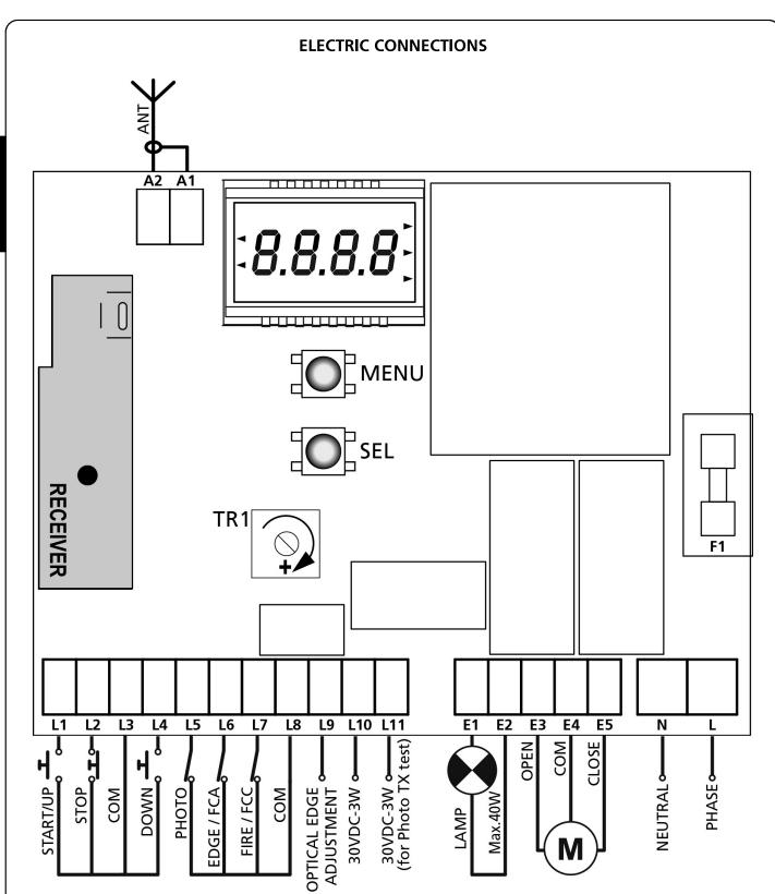
MARNING: Normally closed inputs STOP (L2), PHOTOCELL (L5), EDGE (L6), FIRE (L7), if not used must be bridged through the COMMON terminal (L3 - L8)
