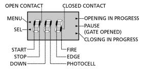
The control panel represents the physical status of the terminal board contacts and of the program mode keys: if the upper vertical segment is on, the contact is closed; if the lower vertical segment is on, the contact is open.
