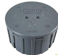
— **In-ground e-Loop** Wireless vehicle detection system uses magnetometer sensors (with optional radar hardware) to detect the presence of oncoming vehicles, these detections are transmitted to a nearby transceiver.
